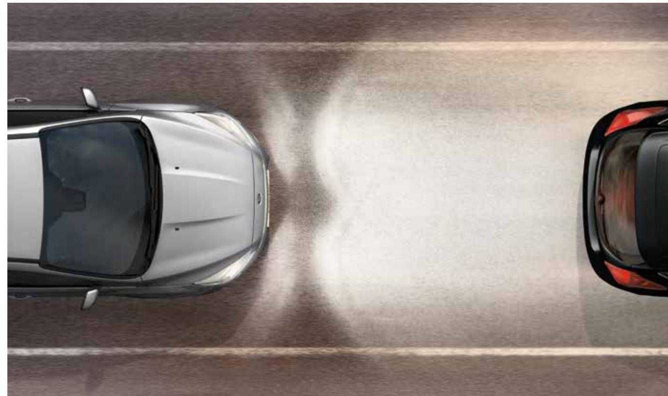
**Active City Stop**<sup>1</sup> automatically applies the brakes if you don't spot the vehicle in front slowing, and works at up to 50 km/h.
